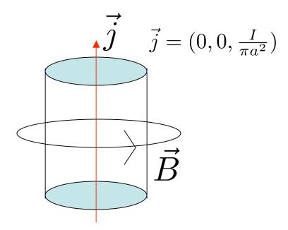
z axis along the wire, r is radial distance from the z axis
