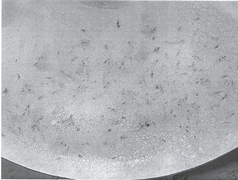
Figure 38. Digital photographs of samples used in carbon fiber thread tests. Here the thread is longer than 3cm and is criss-crossed along the sample.
