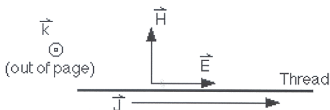
Figure 45. Orientations of the \vec{E} and \vec{H} fields with current flowing along the carbon fiber thread.
