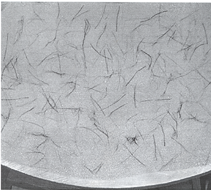
Figure 38. Digital photographs of samples used in carbon fiber thread tests. Here the thread is longer than 3cm and is criss-crossed along the sample.
